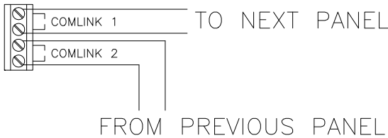
Figure 26: Standard Network Wiring
